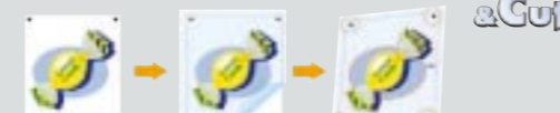
Automatically generates crop marks at the four corners. Allows you to remove the print, laminate and then reload the media. Recalculates the cutting path by adjusting to the crop mark position changes.
